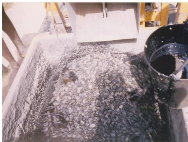
FIG 9: Bitumen being mixed with plastic coated aggregates.
