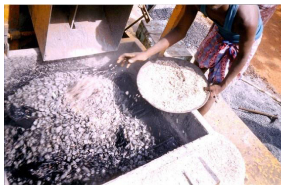
FIG 6: Shredded plastic waste being sprayed over hot aggregates.
